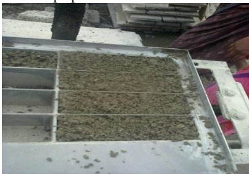
Fig. 2 shake the blend to take out the air with the facilitate of Vibrator apparatus
