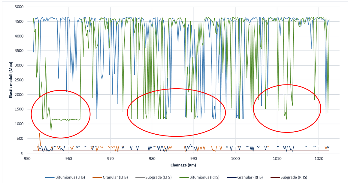
Fig. 3. Elastic moduli of different layers of pavement
