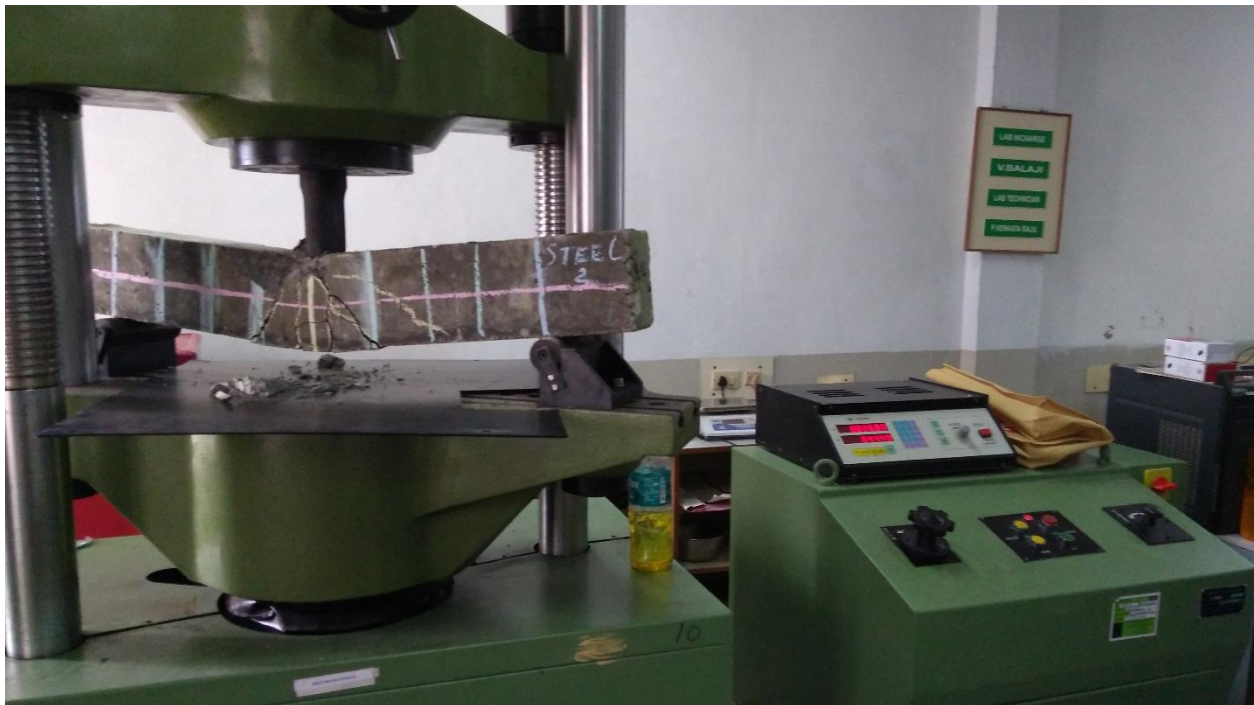
Figure 2- Testing of beam reinforced with steel rebar
