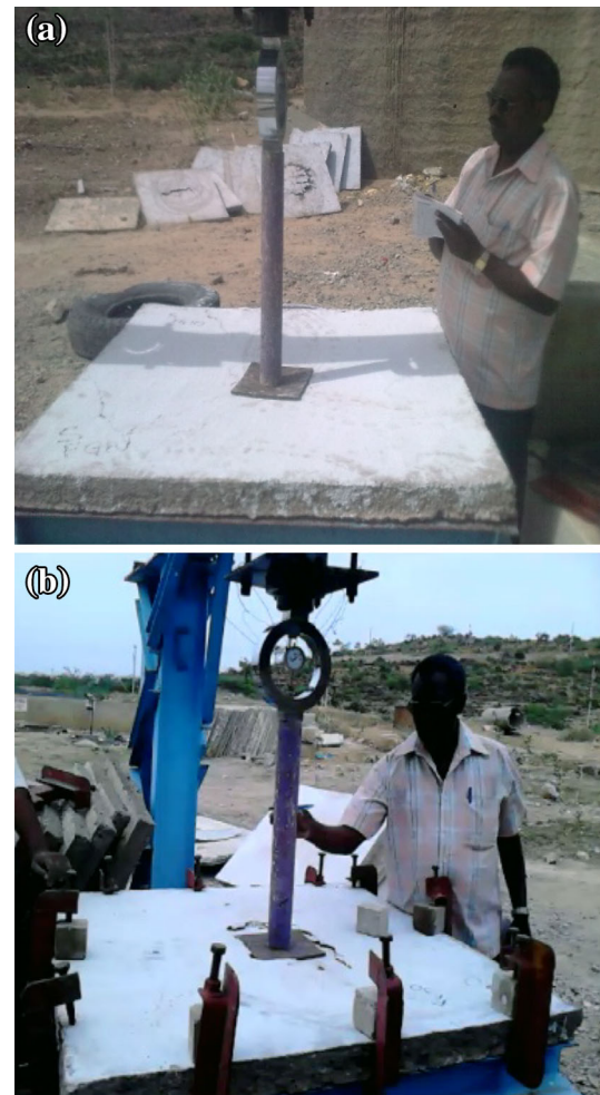
Fig. 1 a Test arrangement for punching shear load of SS slabs. b Test arrangement for punching shear load of fixed slabs
