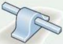
single journal bearing with square shaft
