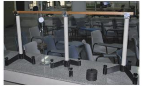
CONTINUOUS BEAM SETUP
