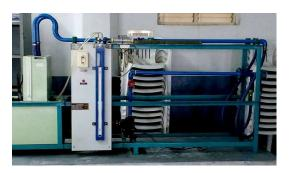
Flow is measured using the differential pressure principle Differential pressure integrated with time, so that it is used to any engineering parameters like flow rate, speed, etc
