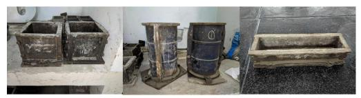
Cube moulds are used for cube testing purpose to find compressive strength of concrete. Cylindrical moulds are used for testing cylinders to find split tensile strength of concrete. Beam moulds are used for testing beam moulds to find flexure strength of concrete specimens
