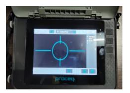
Profometer PM 600 is equipment is used for NDT. This equipment visualizes the diameter of rod, spacing of bars and covers provided in RCC Sections. This equipment is well deserved to identify the reinforcement details at any time after casting.
