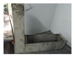
The main objective of this apparatus is to investigate the passing ability of Self Compacting Concrete. It measures the reached height of fresh SCC after passing through the specified gaps of steel bars and flowing within a defined flow distance. With this reached height, the passing or blocking behavior of SCC can be estimated. Two types of gates can be used, one with 3 smooth bars and one with 2 smooth bars. The gaps are 41 and 59 mm, respectively.
