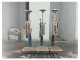
The basic aim is to find out the amount of water content required to produce a cement paste of standard consistency as specified by the IScode and also to check the setting time of cement i.e., both initial and final setting times. Initial setting time test is important for transportation, placing and compaction of cement concrete. Final setting time is the time when the cement
