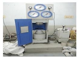
The main objective of this equipment is to determine compressive strength of cement mortar, concrete. Compressive strength results are primarily used to determine that the concrete mixture as delivered on site meets the requirements of the specified strength, fc', in the job specification. Compression strength is the capacity of a material or structure to withstand loads tending to reduce size. Strength of the hardened cement is most important for structural use. This
