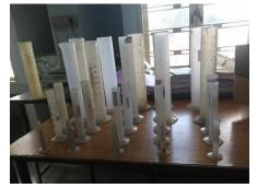
The main objective of measuring jars is to find the percentage of bulking and also to measure amount of water for different tests. Due to bulking, fine aggregate shows completely unrealistic volume. Therefore, it is absolutely necessary that consideration must be given to the effect of bulking in proportioning the concrete by volume. If care is not given to the effect of bulking, in the case of volume batching, the resulting concrete is likely to
