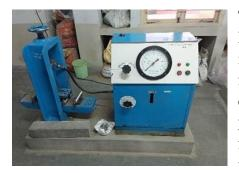
The main objective of this test is to find the modulus of rupture. Flexural strength defined as the stress in a material just before it yields in a flexure test. The transverse bending test is most frequently employed, in which a specimen having either a circular or rectangular cross-section is bent until fracture or yielding using a three point flexural test technique. The flexural strength represents the highest stress experienced within the material at its moment of yield. It is measured in
