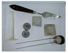
The main aim of this test is to determine the expansion of cement because cement after setting shall not undergo any appreciable change in volume because change in volume after setting causes cracks, undue expansion and as a result disintegration of concrete. In the soundness test a specimen of hardened cement paste is boiled for a fixed time so that any tendency to expand is speeded up and can
