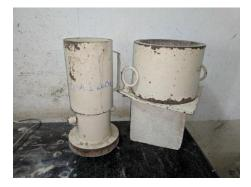
stresses induced by moving vehicles in the form of crushing. With this the aggregates should also provide sufficient resistance to crushing under the roller during construction and under rigid tyre rings of heavily loaded animal drawn vehicles. The aggregate crushing value provides a relative measure of resistance to crushing under a gradually applied compressive load. To achieve a high quality of pavement aggregate possessing low aggregate crushing value should be preferred.
