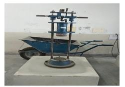
The aggregate impact value indicates a relative measure of resistance of aggregate to sudden shock or an impact, which in some aggregates differs from its resistance to a slope compressive load in crushing test. Toughness is the property of a material to easiest impact. Due to the moving loads the aggregates are subjected to pounding action are impact and there is possibility of stones breaking into smaller pieces. Therefore a test design to
