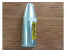
The main objective of this apparatus is to assess the likely compressive strength of concrete with the help of suitable co-relations between rebound index and compressive strength, uniformity of concrete, assess the quality of concrete in relation to standard requirements, assess the quality of one element of concrete in relation to another. This is a simple, handy tool, which can be used to provide a convenient and
