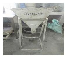
The main objective of V-funnel flow time is the period a defined volume of Self Compacting Concrete needs to pass through a narrow opening and gives an indication of the filling ability of SCC provided that blocking and/or segregation do not take place; the flow time of the V-funnel test is to test degree related to the plastic viscosity. The V-funnel flow time  $T_V$  is the period from releasing the gate until first light enters the opening, expressed to the nearest 0.1 second
